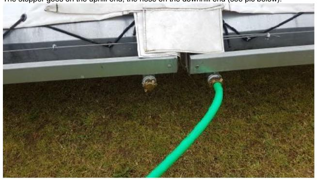
The hoses go on the bottom end of cover and should be run off the square with the slope where possible.
